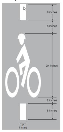
Figure 17 – Shared Lane Pavement Markings
